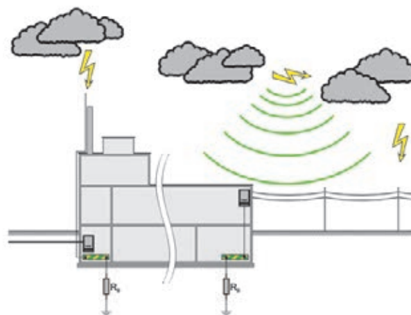
Surge currents exceeding 200 kA can be generated by cloud-to-ground but also cloud-to-cloud lightning discharges.
